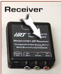
4. Connect the “Receiver” to the display device (e.g. LCD TV or Projector). Make sure to match the colors of the YPbPr cables to your display’s input port.
