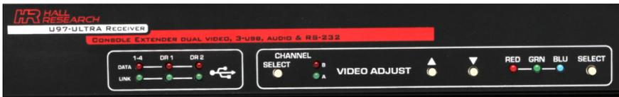
In RUN-mode, all LEDs and buttons for video adjust are off. And tapping on the control buttons have no effect. This prevents accidental and unintended video adjustment, though it is possible to make adjustments in RUN mode by long pressing the Select button as described below.
